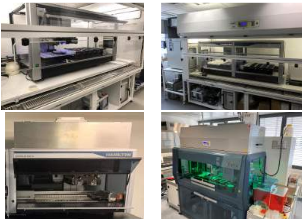
Figure 14: Four Examples of System Configurations Ensuring Sterility of the Automated Workflow. The two upper photos show Hamilton systems inside Class II BSCs, and the two lower photos show Hamilton systems with HEPA Hoods. Photos were taken by Hamilton Application Specialists during system installations.
