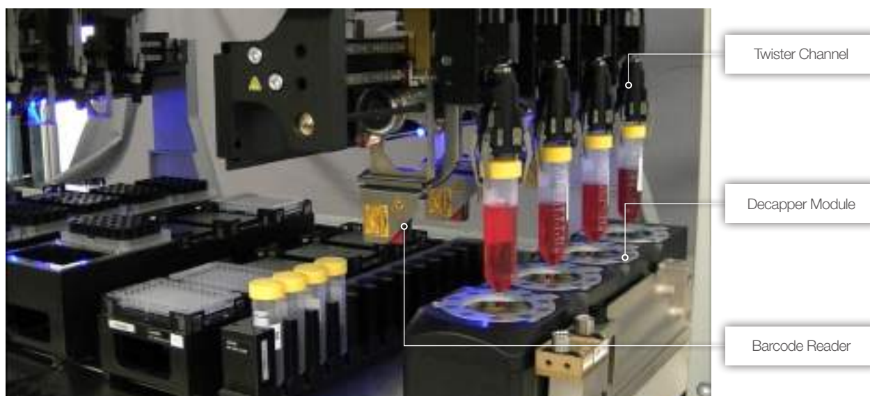
Figure 9: Twister Channel and Decapper Module Integrated into Hamilton Automated Platforms.
