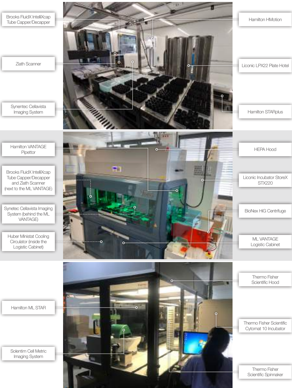
Figure 16: Three Examples of Integrations of Hamilton platforms with Third-party Instruments for Cell-Related Assays. Photos were taken by Hamilton Application Specialists during system installations.
